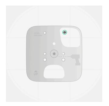
9. Remove the Superior SeismoProtect G3 Fibra lid and drill holes for the cable. When using the bundled armored cable, carefully break out the perforated part to bring the cable out. When using other cables with smaller diameters, drill holes for the cable at low speeds.
