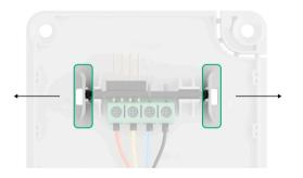
3. Prepare holes for cable output in advance. To output cables from the back of the keypad, break out the perforated part on the SmartBracket mounting panel. To output cables from the bottom of the keypad, make holes in the bottom of the enclosure using a drill bit, a special milling cutter for small holes, or handcutting tools.
