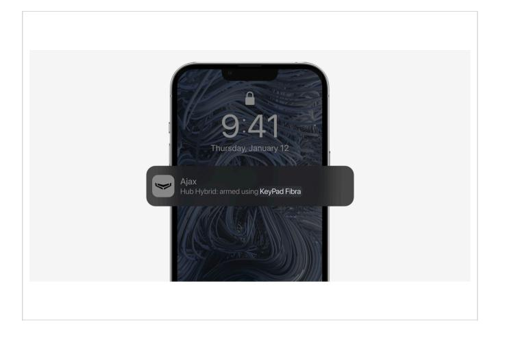
KeyPad Fibra is locked for the time specified in the settings if an incorrect password is entered three times in a row within 1 minute. The corresponding notifications are sent to users and to the monitoring station of the security company. A hub administrator or PRO with administrator rights can unlock the keypad in the Ajax app.
