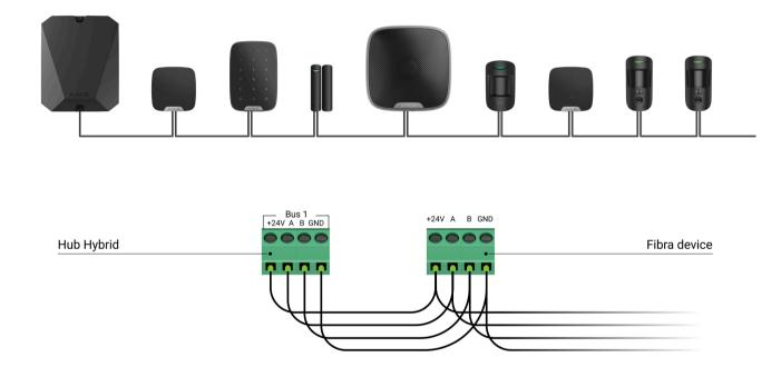
For the **Beam** (**Radial**) topology, be sure to install a 120 Ohm terminating resistor at the end of the line (included in the hub complete set). The terminating resistor is connected to the signal terminals of the last detector on the line.
