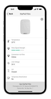
The states include information about the device and its operating parameters. The states of KeyPad Fibra can be found in the Ajax app:
