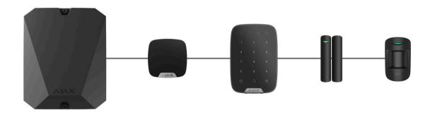
**Ring connection method** occupies two Fibra lines of the hub. If the ring breaks in one place, no device will be disabled. The ring reconfigures into two lines, which continue to operate normally. Users and the security company will receive notification about the break.
